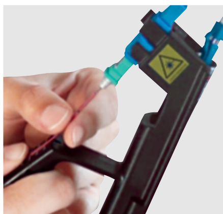
Insert the fibre in the connector
