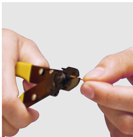
Remove the sheath from the fibre
